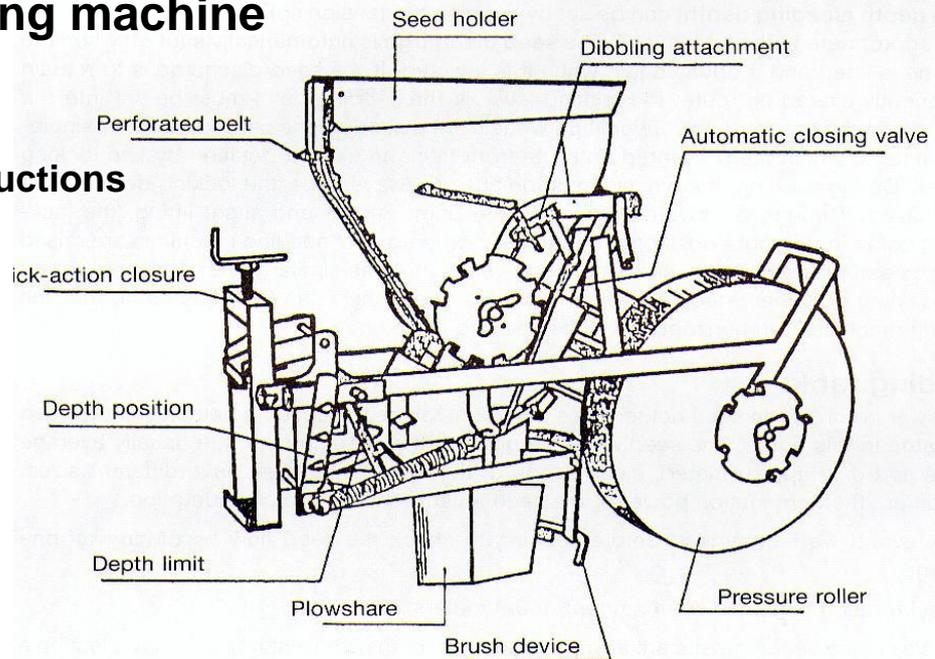
**Before starting to sow**, the machine must be lubricated on all moving parts. The V belt only has to be loosely tightened, since slipping is not to be feared even if the V belt is slack. If it is necessary to retighten the V belt, the nut of the V belt disk on the seed box must be removed. When the washers between the V belt disk halves are removed, the belt can be adjusted to the desired tautness.
