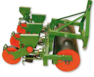
The tool carrier with the roller is particularly recommended for pre-rolling of loose soil to achieve an even seed depth.
