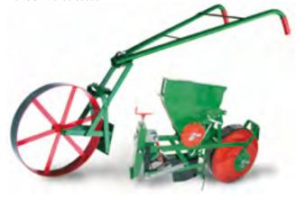
The undercarriage turns the GSD into a single-drill hand pushed seeder suitable for areas which are too small or too difficult to access for a multiple-row device (i.e. head lands or small field corners).
