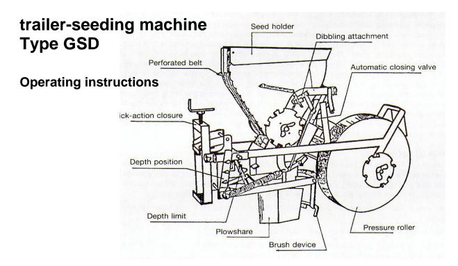
**Before starting to sow**, the machine must be lubricated on all moving parts. The V belt only has to be loosely tightened, since slipping is not to be feared even if the V belt is slack. If it is necessary to retighten the V belt, the nut of the V belt disk on the seed box must be removed. When the washers between the V belt disk halves are removed, the belt can be adjusted to the desired tautness.
