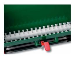
Sowing takes place via a **Nylon brush**. The adjusting lever serves infinitely variable opening of the bottom run-off plate.
