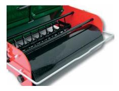
The dibbler is set to transport position by operating the **bracket**.
