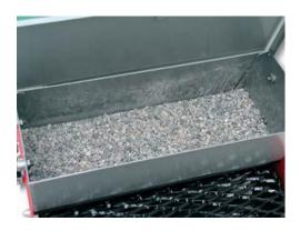
A detachable, robust **weight box** that can be filled with various minerals (sand, stones) is located above the flat pressure roller.
